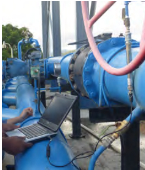
Figure 13: Pressure measurement using a portable electronic pressure sensor (Photo: CAH, 2015)
