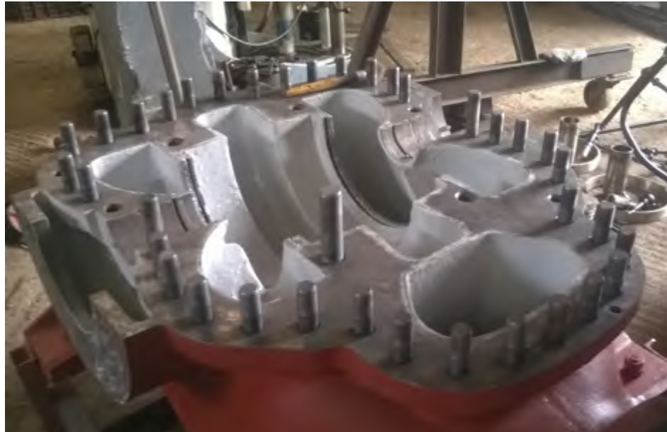
Figure 37: Newly painted pump casing (photo: Morocco, 2015)
